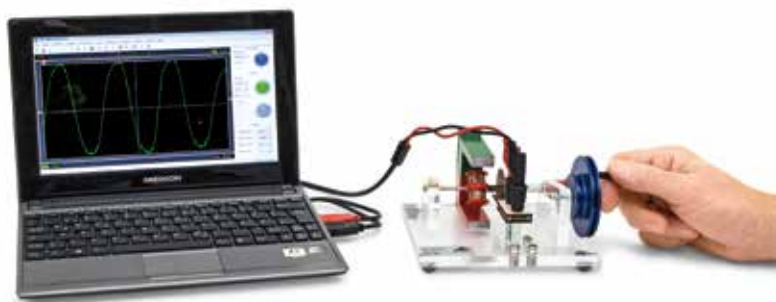
Operating as an AC generator
