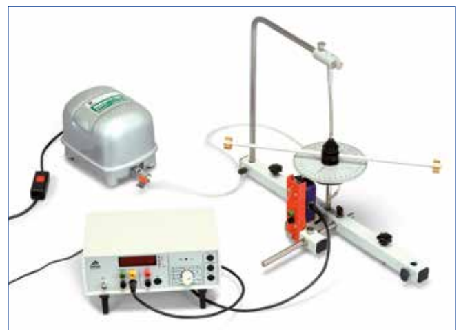
Measuring the period of oscillation and determining the moment of inertia
