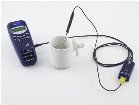
Fig. 1: Experimental demonstration of Newton's law of cooling
