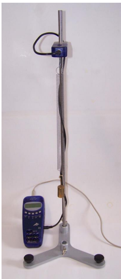
Fig. 1 Measuring the oscillations of a weakly-damped mass-and-spring system
