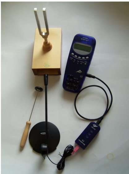
Fig. 1: Measuring the sound wave of a tuning fork
