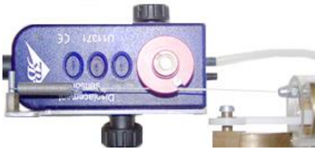
Fig. 2 Attachment of the thread to displacement sensor pulley
