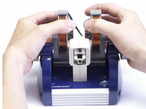
Fig. 4 Pulling the two permanent magnets apart
