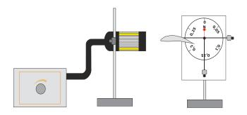
4.3 Using the component scale to measure the drag force on a disc
