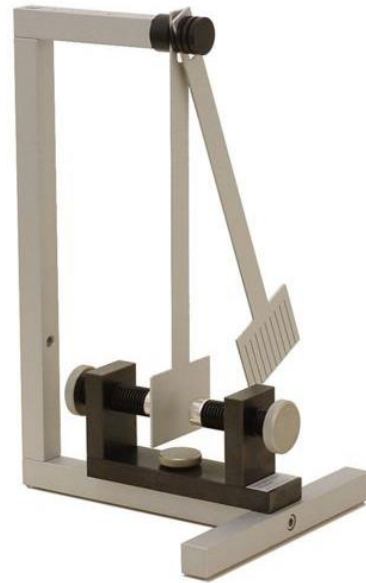
Fig. 5 Experiment set up for "induced eddy currents"
