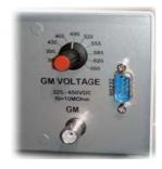
RS232 interface to PC für PC GM BNC-connector for Geiger-Müller tube **GM VOLTAGE** Voltage regulation potmeter for the Geiger-Müller tube.
