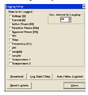
Here it is possible to mark each data that is to be logged, and at what interval. The more data to log at each interval, - the fewer "log-lines" are possible. For maximum number of intervals ("log-lines"), select only the data that is necessary. The maximum number of log-lines and the maximum logging-time is calculated and displayed.
