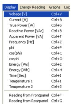
This is where to select what is displayed on the digital LED-display, and if measurements are made on the front panel or on the rear panel.
