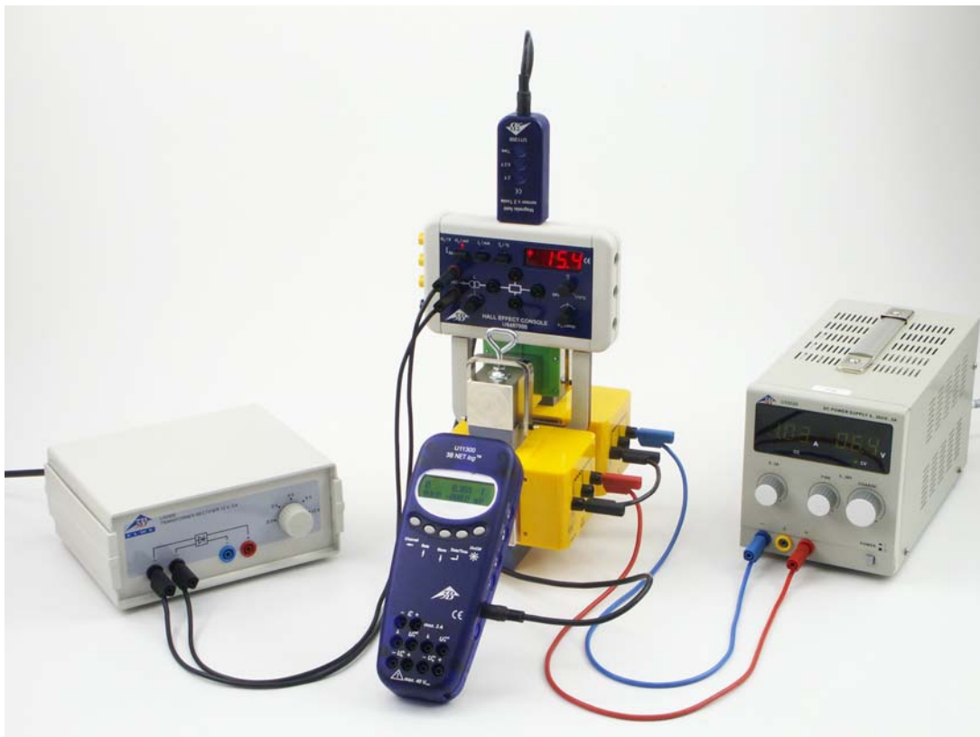
Fig. 1 Measurement of flux density in the air gap between pole pieces of an electro-magnet in an experiment set-up using the basic Hall-effect apparatus
