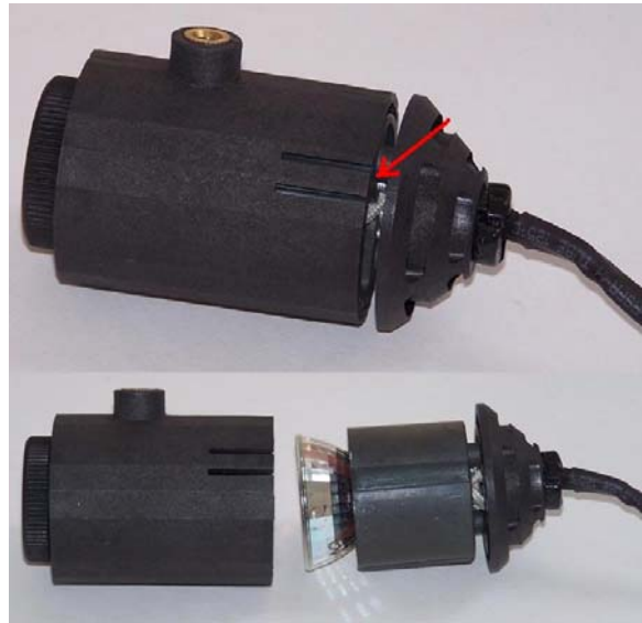
Fig. 1 Changing the bulb in the top light
