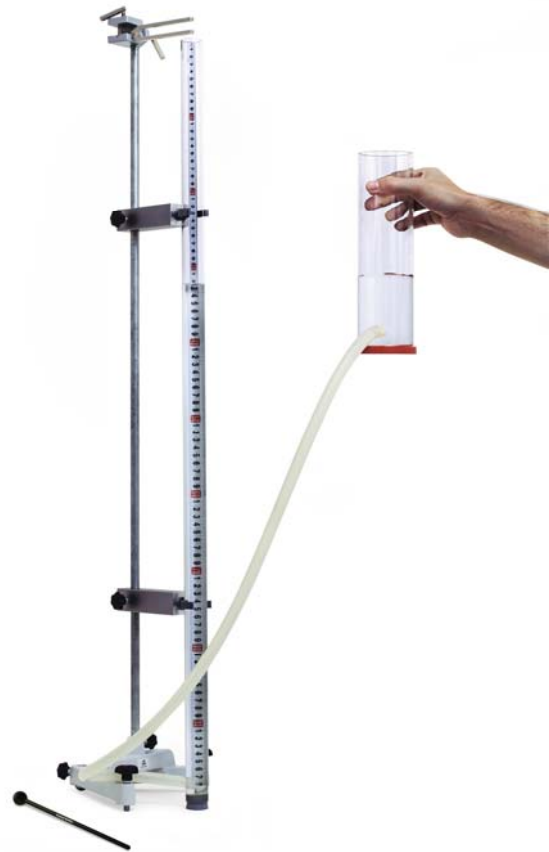
Fig. 1: Quincke's resonance tube in operation.
