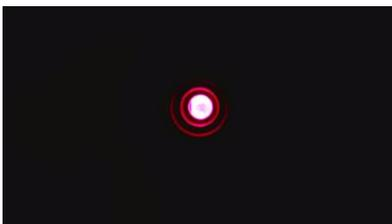
Fig. 7 a: First convex lens positioned and fixed in place at 232 mm on the optical bench (cf. Fig. 4 d). Stepped hole and spot appear enlarged, but do not fill the screen.
