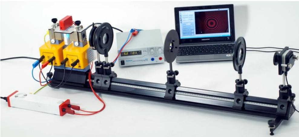
Fig. 1: Measurement arrangement for the longitudinal Zeeman effect
