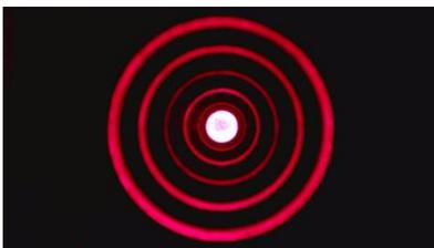
Fig. 6 e: Camera module pushed along the optical bench so far from the electromagnet that the image of the stepped hole fills the screen
