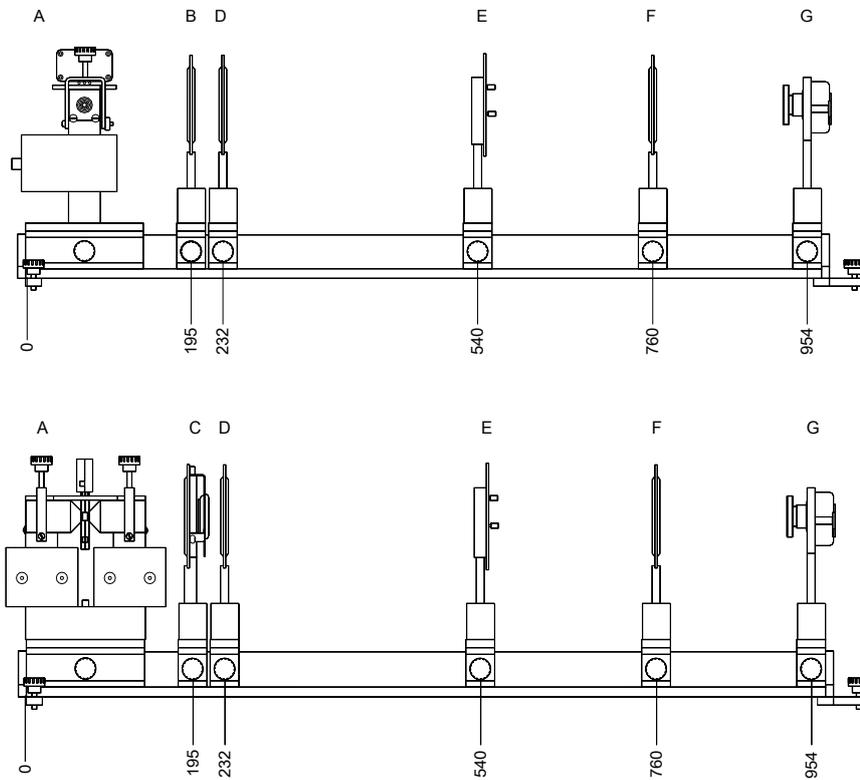
Fig. 4: Equipment set-up for the longitudinal (bottom) and transversal (top) Zeeman effect. A: Electromagnet with Cd lamp, B: Polarisation filter, C: Quarter-wavelength plate with polarising attachment, D: First convex lens  $f=100$  mm, E: Fabry-Pérot etalon, F: Second convex lens  $f=100$  mm, G: Camera module
