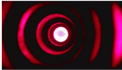
Fig. 6 b: Adjustment error: Electromagnet skewed. The stepped hole does not appear concentrically.
