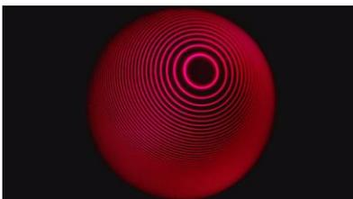
Fig. 9 e: Adjustment error: Etalon tilted. Correction: Reposition using the three adjustment screws in the housing.
