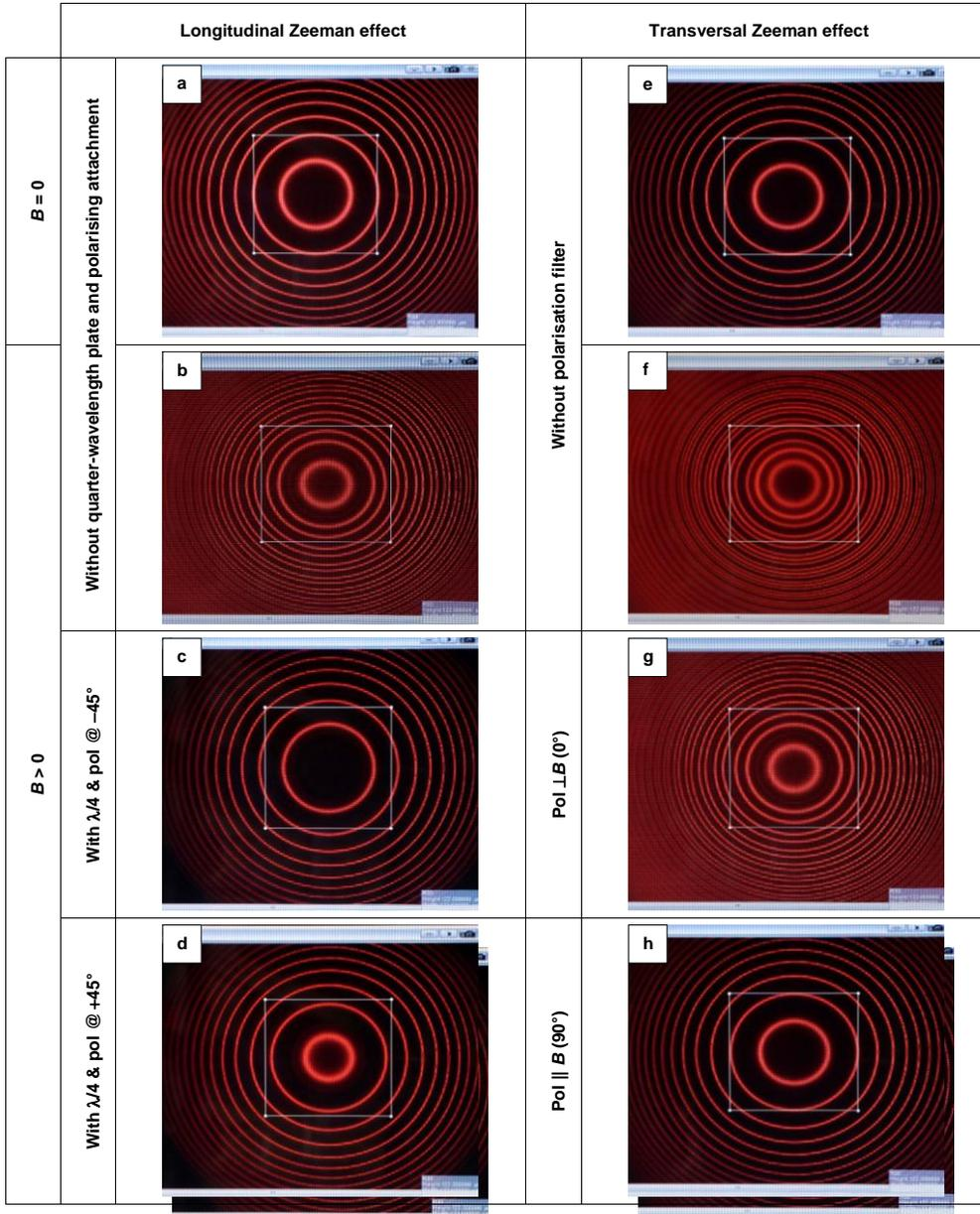
Fig. 10: Observation of the doublet and triplet splitting of the red cadmium line in an external magnetic field and investigation of polarisation, screenshots from the camera software. As an orientation aid, the second interference ring from the centre is indicated with a frame.
