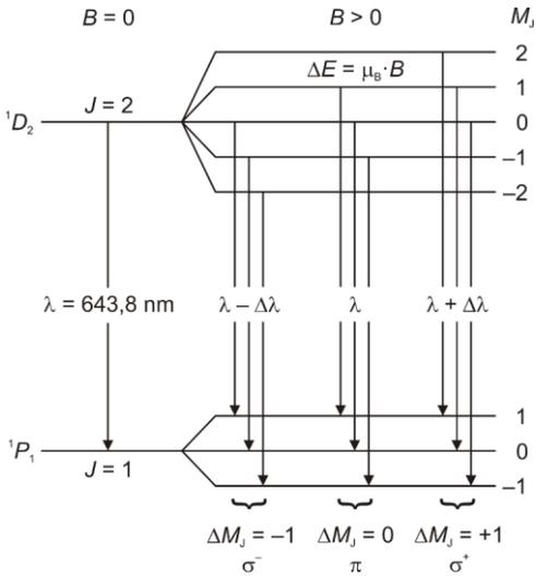
Fig. 2: Normal Zeeman effect in the red spectral line of cadmium. Splitting of energy levels and transitions permitted according to the selection rules for electrical dipole radiation.
