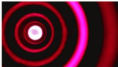
Fig. 6 d: Adjustment error: Camera module skewed in the optical slider
