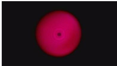
Fig. 9 b: Adjustment error: Poor focus
