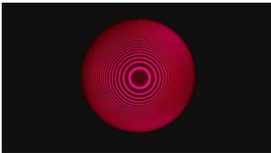
Fig. 9 a: Fabry-Pérot etalon positioned and fixed in place at 540 mm on the optical bench (cf. Fig. 4 e), interference rings appear in sharp focus.
