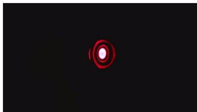
Fig. 7 b: Adjustment error: Convex lens skewed in the optical slider
