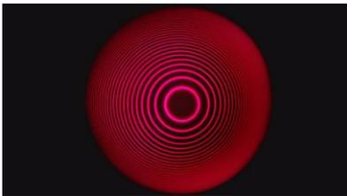
Fig. 9 c: Second convex lens pushed towards the camera module so the interference rings fill the screen. Focus adjusted accordingly.
