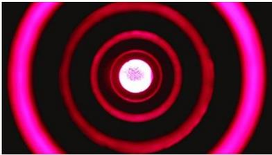
Fig. 6 a: Camera module positioned directly in front of the electromagnet. Stepped hole of the pole piece and Cd lamp spot appear concentric and centred. Focus on the spot.
