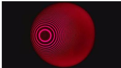
Fig. 9 d: Adjustment error: Etalon skewed in the optical slider.
