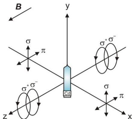
Fig. 3: Polarisation of electrical dipole radiation depending on the direction of travel
