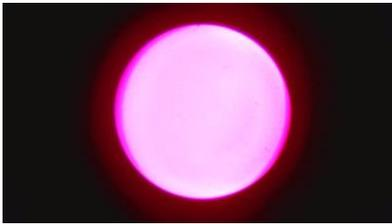
Fig. 8 a: Second convex lens positioned and fixed in place at 760 mm on the optical bench (cf. Fig. 4 f). The spot appears enlarged and nearly fills the screen.
