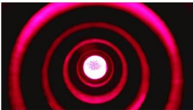
Fig. 6 c: Adjustment error: Camera module set too high in the optical slider
