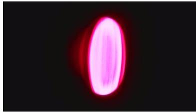
Fig. 8 b: Adjustment error: Convex lens skewed in the optical slider
