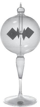
The Crookes radiometer is used for demonstrating the conversion of radiation energy into kinetic energy.
