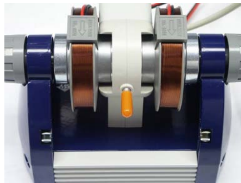
Fig. 4 Basic unit with DPPH sample inserted
