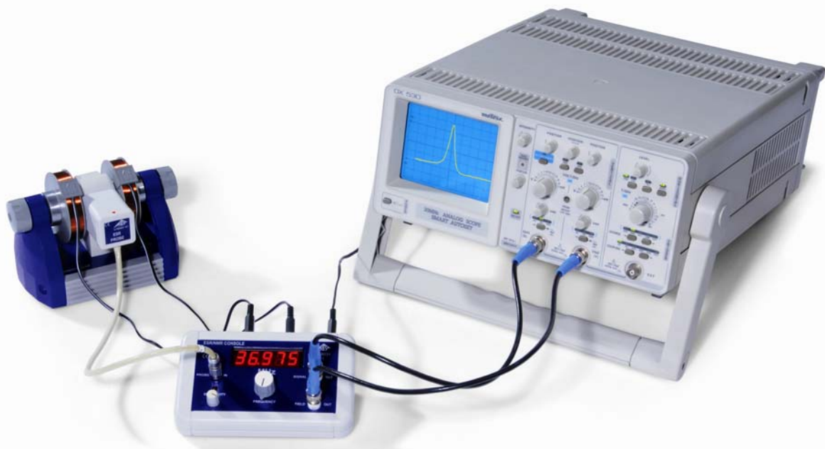
Fig. 5 ESR experiment set-up using an oscilloscope
