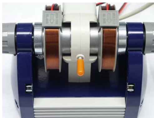
Fig. 4 Basic unit with DPPH sample inserted
