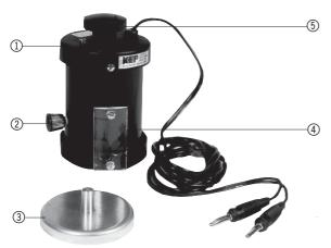
The single-beam lamp is used in experiments to demonstrate geometric optics on magnetic boards (U14600).
